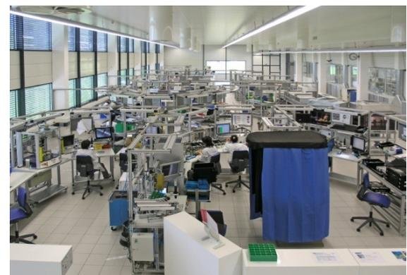
The size of parts and the required precision necessitate a controlled atmosphere in the entire assembly workshop, with continual air change and filtration. A clean room ISO 7 is available for implantable medical applications.
