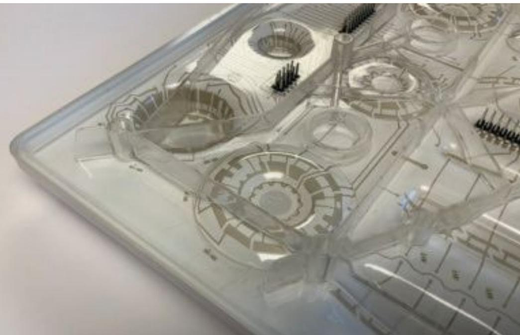
Speaking of LEDs, adding them to IME parts can produce attractive, uniform backlighting to differentiate products from the competition. When printed with transparent ink, for example, an icon can look like it's glowing. The look is accomplished with the use of side firing LEDs and manipulating the resin system to work as a light guide.
