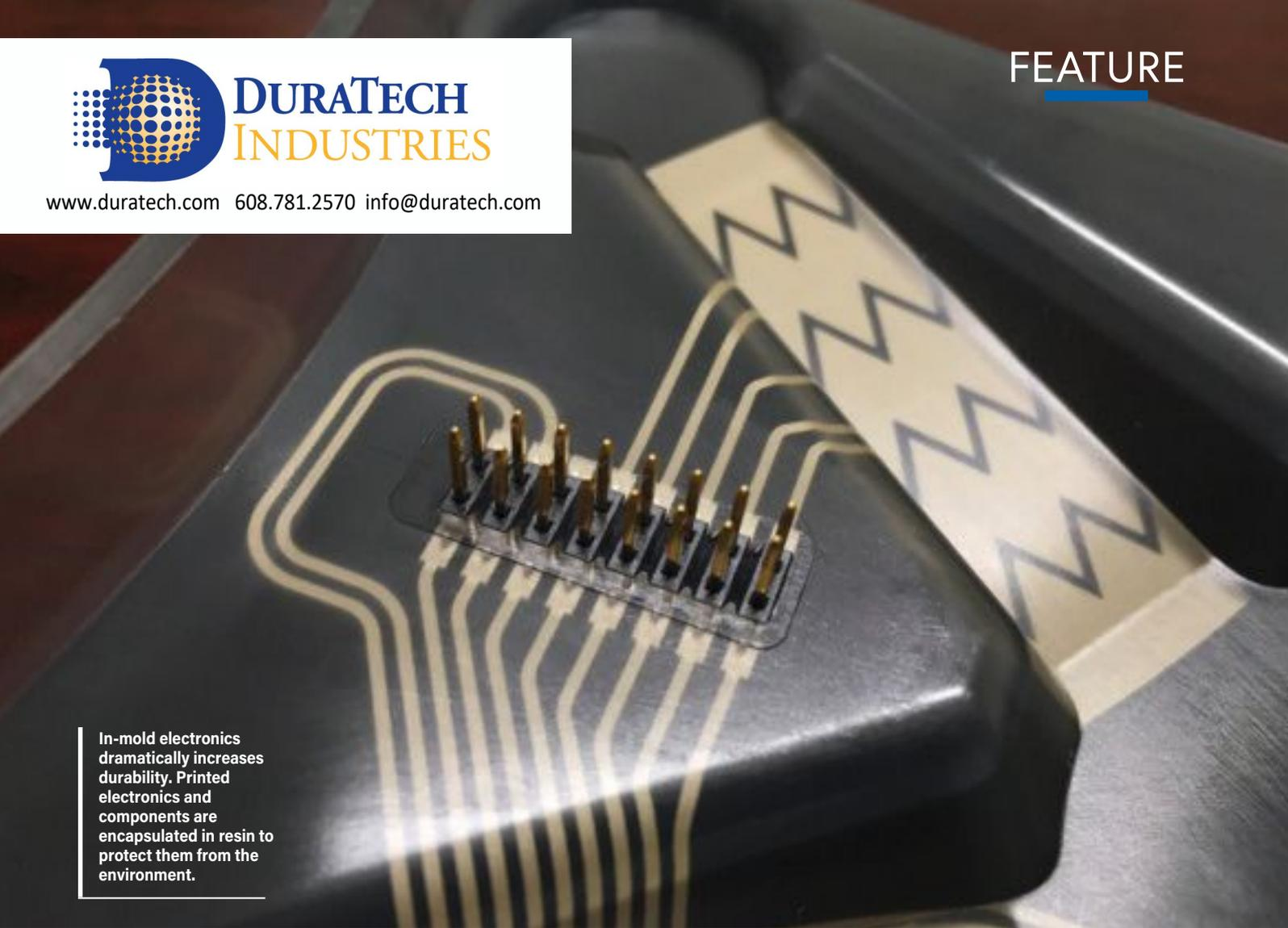
In-mold electronics dramatically increases durability. Printed electronics and components are encapsulated in resin to protect them from the environment.
